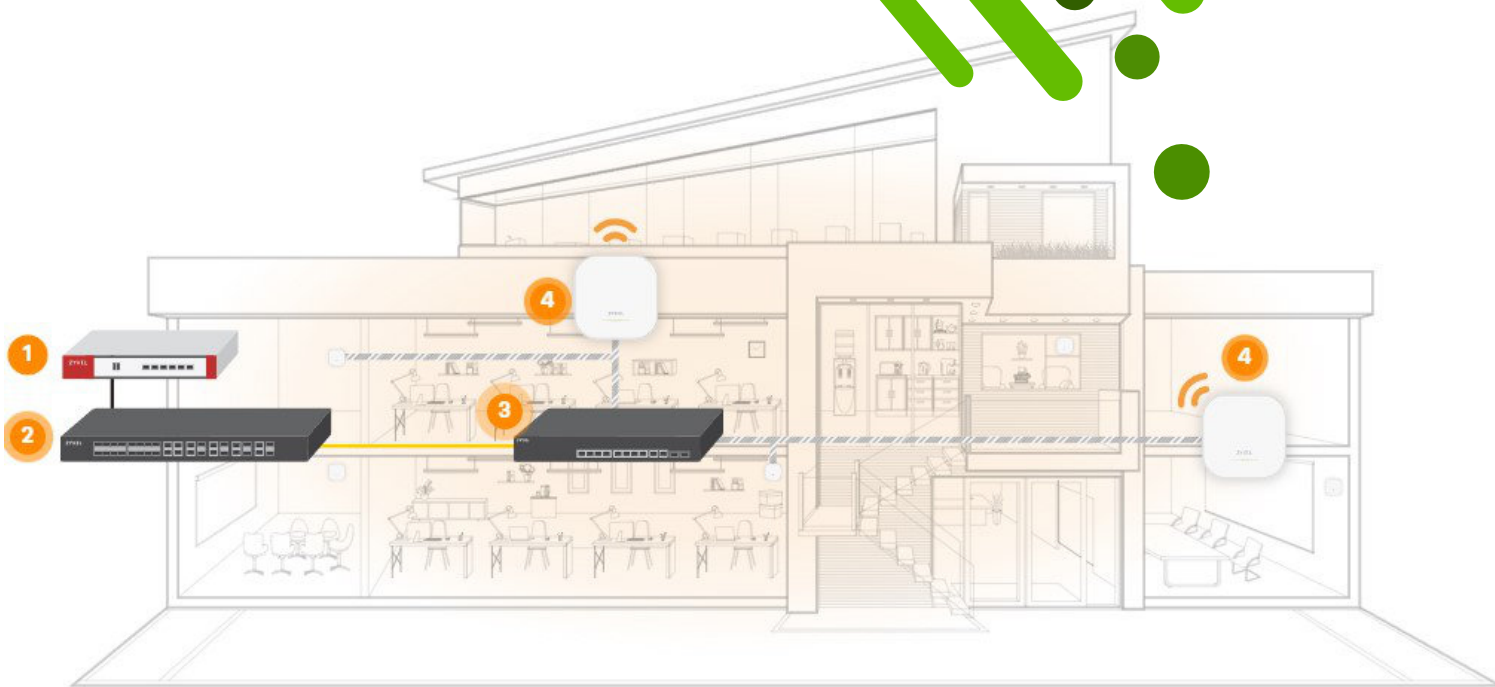
1. Security Firewall 2. L3 Aggregation Switch 3. Multi-Gigabit POE Switch 4. Wifi 6E Access Point
